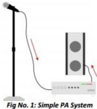
Fig No. 1: Simple PA System
